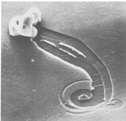
**Figure 12** Movement of molybdenum carbide particle on graphite basal plane after heat-treatment at 2525° C,  $\times 4000$ .
